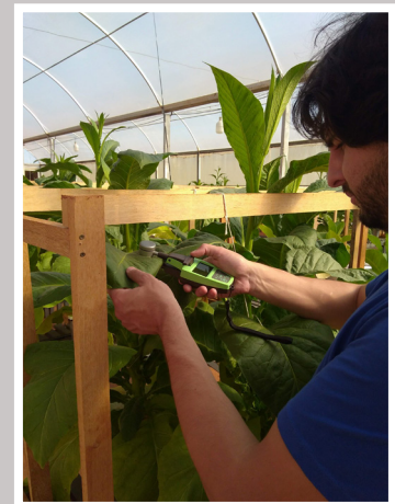
Measuring chlorophyll, flavonols and anthocyanins in tobacco leaves with the optical sensor Dualex
