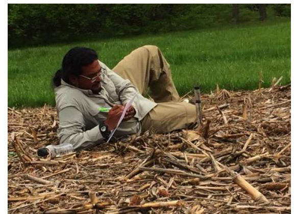
Above: Nall measuring water infiltration in the field using a portable mini-disk infiltrometer.
