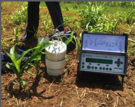
Measuring GHG emissions in the field using a photoacoustic infrared spectroscopy multi-gas monitor.
